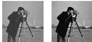
Fig. 3. Left: Noisy image ( \sigma = 20 , PSNR = 22.10 dB). Right: Denoised image (PSNR = 30.06 dB) using OCTOBOS ( K = 4 ).
